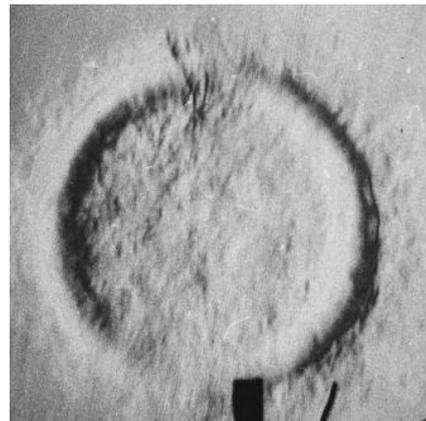
Fig.1. Turbulent vortex ring (front view)
