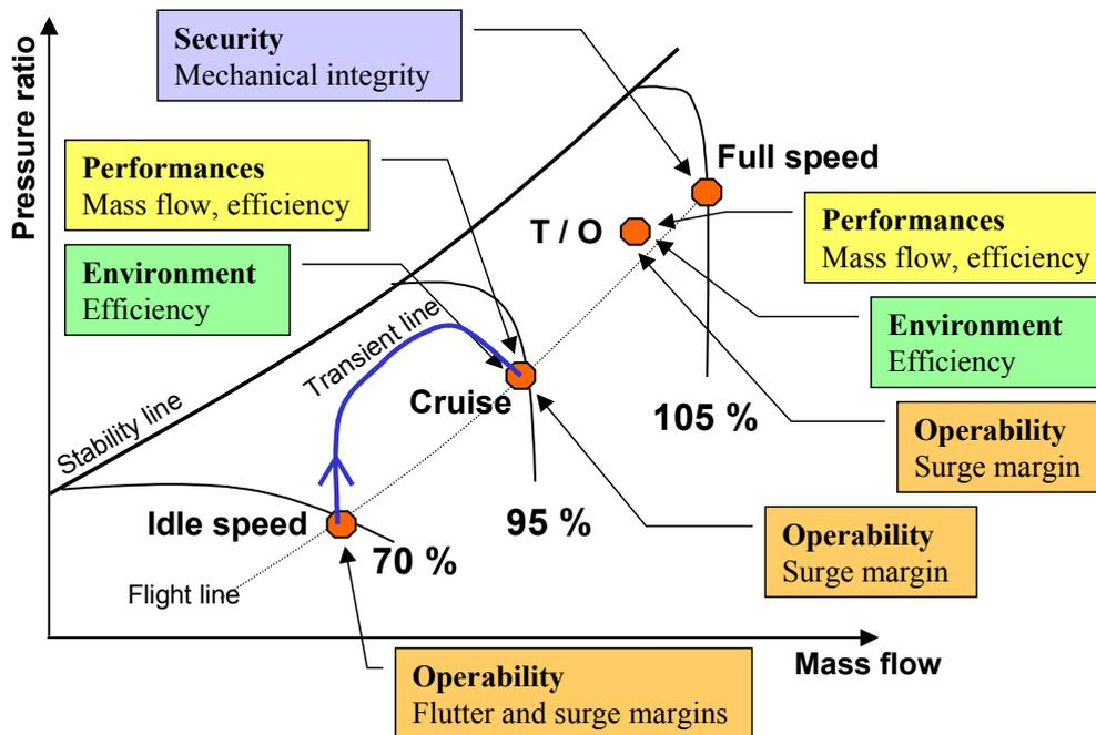
Fig. 1 - Compressor map and design objectives
