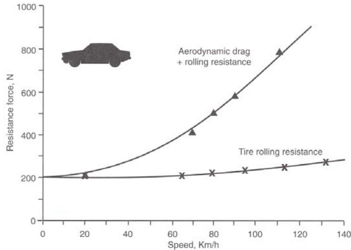
Figure 1. Aerodynamic drag + rolling resistance as function of driving speed for a typical sedan, from Barnard [1].
