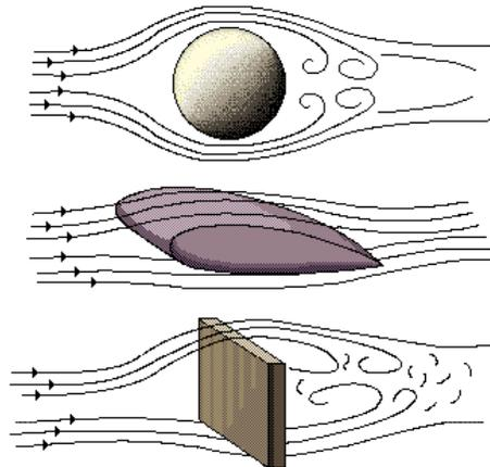
Figure 2 Three fundamental flow cases.
