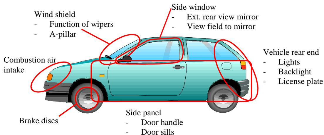
Fig. 1: Areas on a passenger vehicle critical to soiling.
