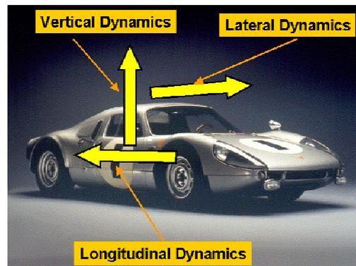
Fig 1.2: Components of vehicle dynamics
