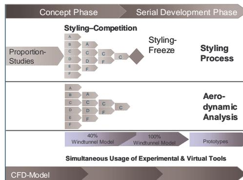
Fig.1: CFD in the aerodynamic development process [1]
