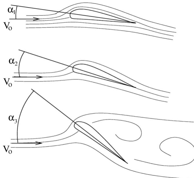
*Figure 1: Sketch of flow past airfoil at increasing angles of attack*
