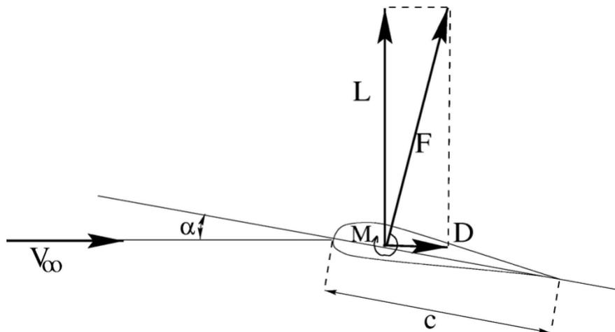
Figure 2: Definition of lift and drag
