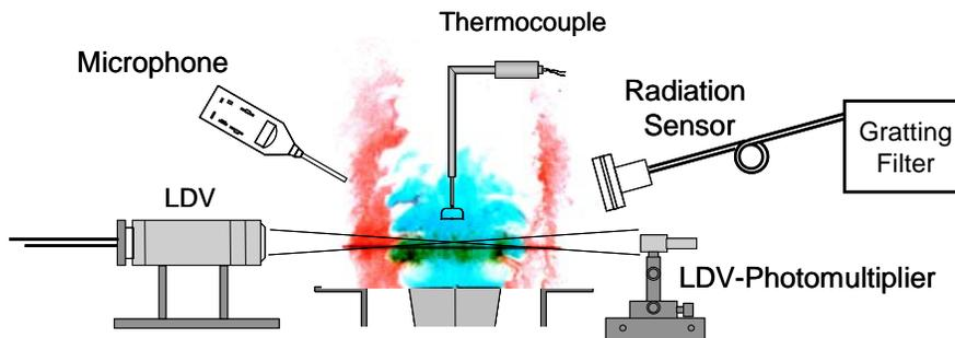
*Figure 1.1. Schematic diagram of combination between LDV, Microphones, Fine-wire thermometry and Radiation sensor to characterize an unsteady flame*
