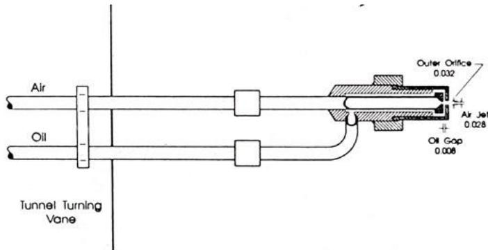
Figure 1: Scheme of a particle generator based on an oil/air atomiser.
