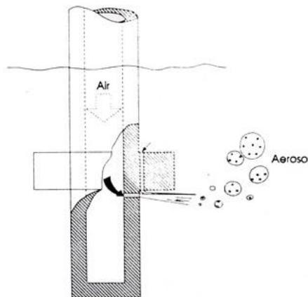
Figure 2: Scheme of Laskin nozzle device
