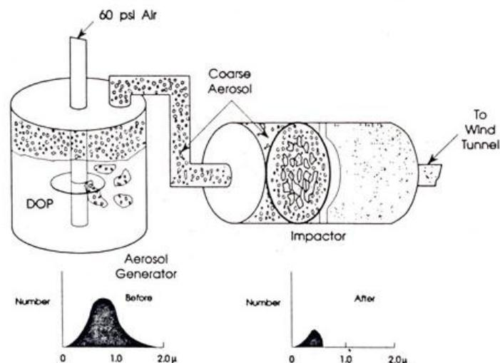
Figure 3: Scheme of a Laskin vaporisation system with an impactor [1]
