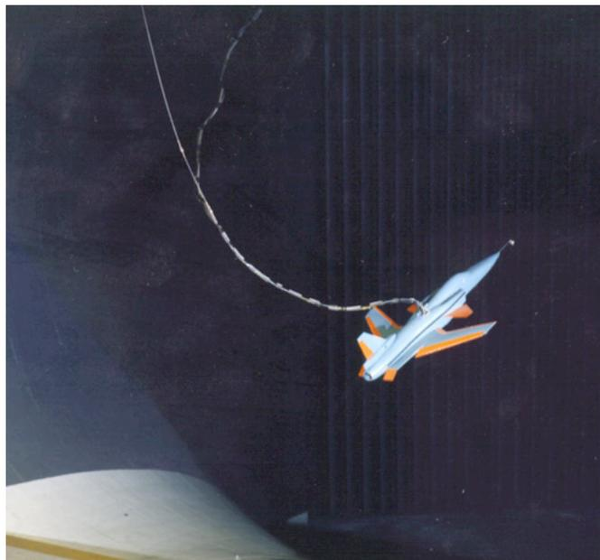
X-29 free-flight model in the NASA Langley Full-Scale Tunnel
