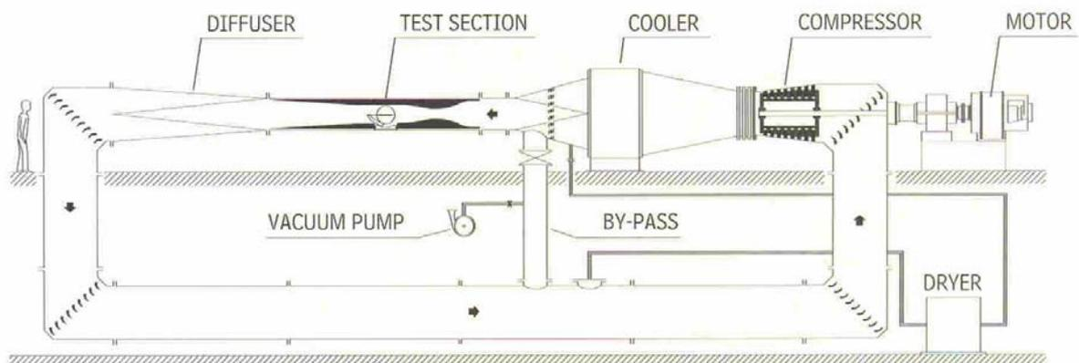
The VKI-S1 wind tunnel is a continuous closed circuit super/trans/sub-sonic wind tunnel of the Ackeret type and driven by a 615 kW axial flow compressor. Two 40 cm x 36 cm test sections are available. A transonic test section with adjustable slotted
