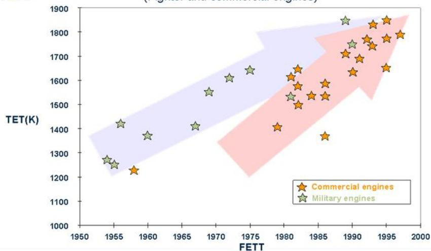
Figure 3 - Turbine inlet temperature evolution
