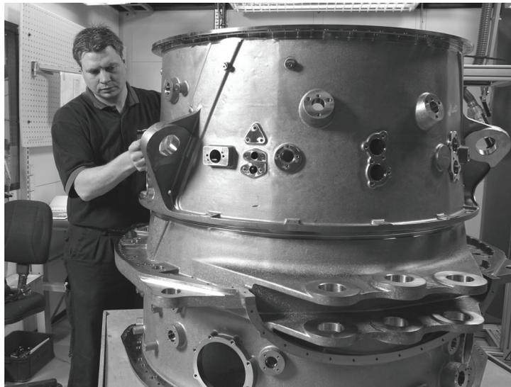
Figure 1. An aircraft engine titanium structure made by vacuum investment casting technology. The intermediate compressor casing for the R&R Trent 900 engine.
