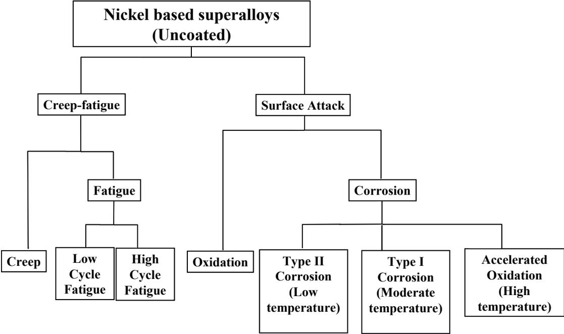
Figure 2 Failure Modes of Uncoated Components
