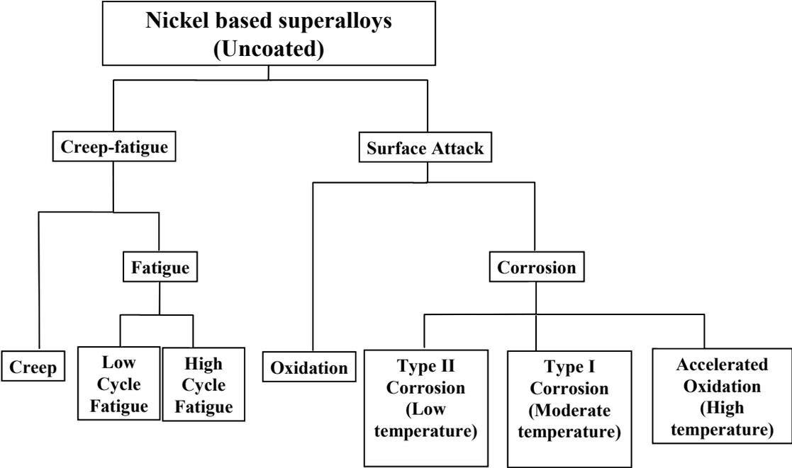
Figure 2 Failure Modes of Uncoated Components
