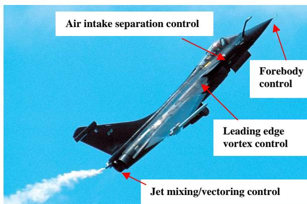
Figure 1 : Various flow controls on a fighter
