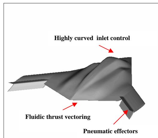
Figure 2 : Various flow controls on a UCAV
