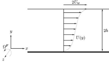
Figure 1: Plane turbulent Couette flow seen from a reference frame which rotates about the spanwise  $z$ -axis. The typical  $S$ -shaped mean velocity profile  $U(y)$  is indicated.
