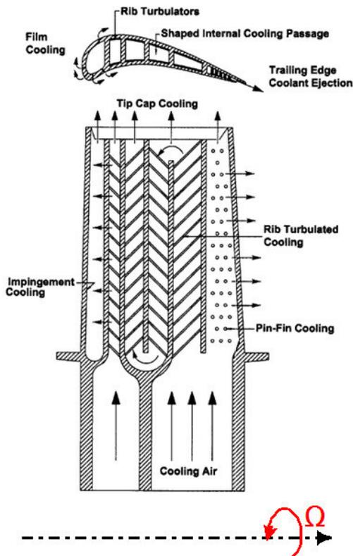
Figure 1 Typical internal blade-cooling arrangements. From Fu et al. (2005)
