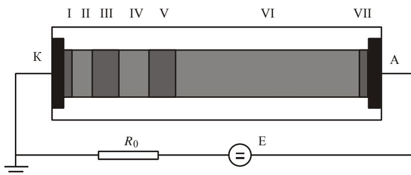
Fig. 2. The scheme and structure of classical glow discharge: I – Aston dark space; II – Cathode luminescence; III – Cathode dark space; IV – Negative luminescence; V – Faraday dark space; VI – Positive column; VII – Anode dark space; K – Cathode; A – Anode;  $R_0$  – Ohmic resistance of external circuit; E – Voltage of power supply
