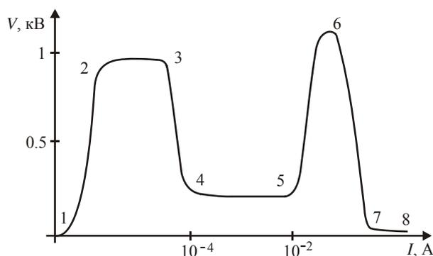
Fig. 1. The diagrammatic representation of Voltage-current characteristic of electric discharges (boundary values of Voltages and currents are approximate): 1-2 – area of non-self-maintained discharge; 2-3 – dark the Townsend discharge; 4-5 – normal glow discharge; 5-6 – anomalous glow discharge; 6-7 – area of transition from glow to arc discharge; 7-8 – arc discharge
